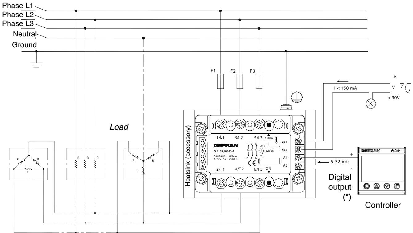
\* Only in the version with option overtemperature alarm output
