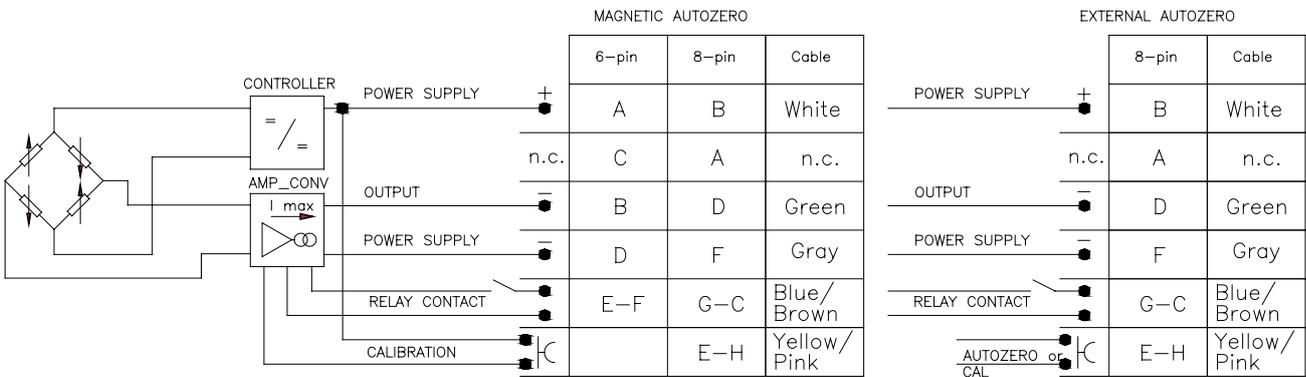
The cable shield is tied to both sides, i.e. to the sensor connector and to the controller
