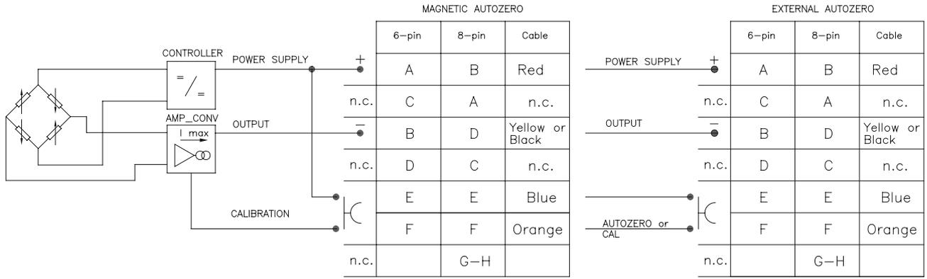
The cable shield is tied to both sides, i.e. to the sensor connector and to the controller
