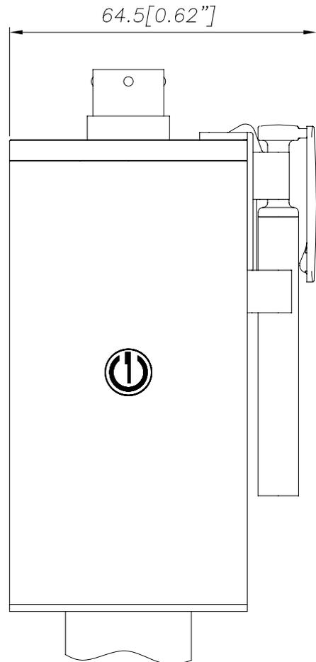
The Autozero function is activated through a magnetic contact (external magnet supplied with the sensor).
