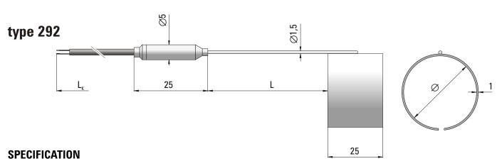
Application temperature measurement of solid surfaces, parts of machinery
